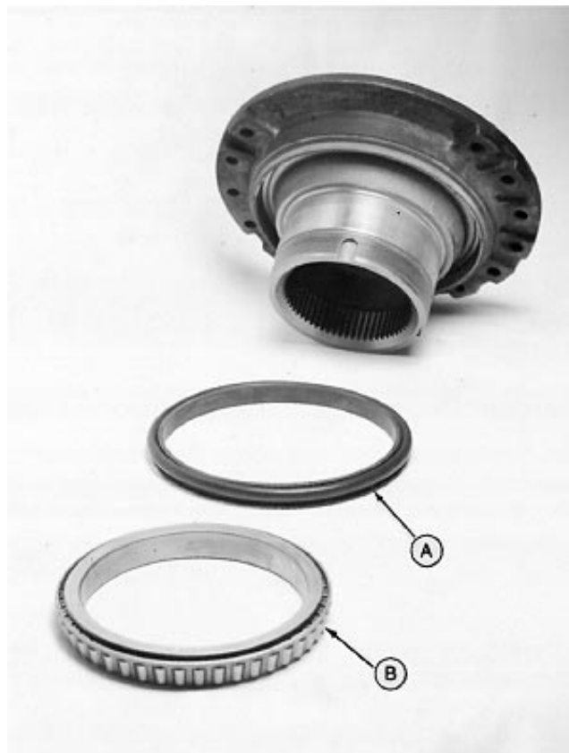
A—Metal Face Seal B—Bearing Cone
