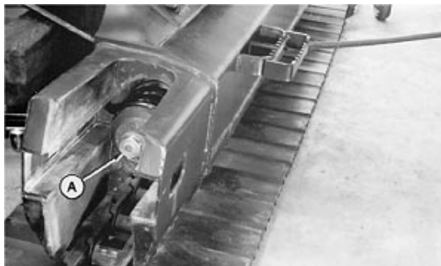
A—Track Adjuster Cylinder and Recoil Spring
