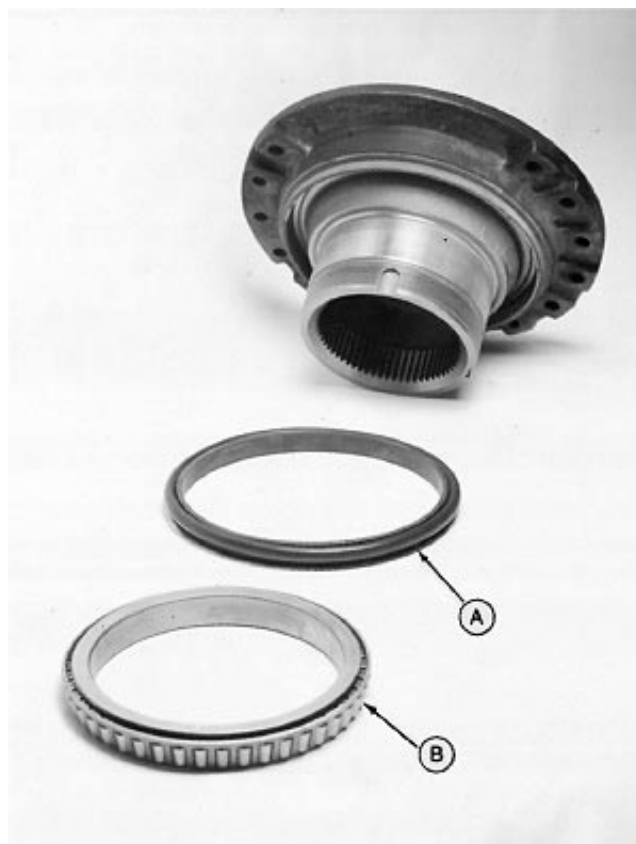
A—Metal Face Seal B—Bearing Cone
