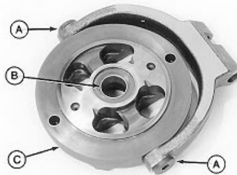
A—Pivot Plug (2 used) B—Bushing C—Valve Plate
