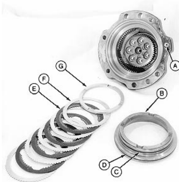
A—Brake Port B—Piston C—O-Ring D—O-Ring E—Disk (4 used) F—Plate (5 used) G—Spacer
